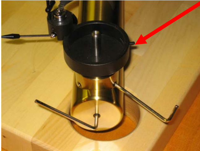
The bearing base with cable holder in its brass pillar on Stabi S. Fig. 2
